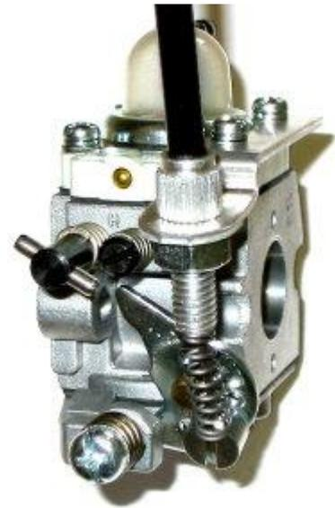
HP carb with throttle bracket attached, throttle barrel and nut installed, spring installed over the throttle cable, and the end of the cable connected to the swivel. Your carb should look like this before you bolt it on.
