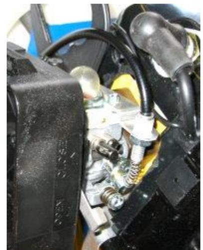
Air filter, carb, and gasket are now connected to the manifold.
