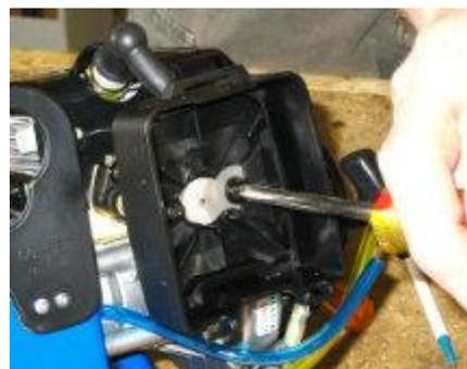
Unscrew the bolts that hold the air filter and carburetor on.
