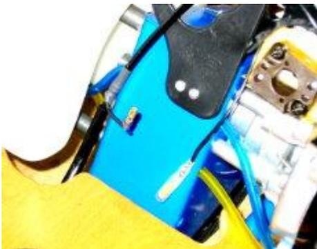
The throttle cable has been moved to the gas tank side.
