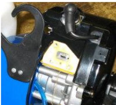
The insulator manifold is removed in this picture.
